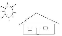
What paint should be used for minimum heat gain during summer ? White Paint  $\epsilon$  short wave = =  $\alpha$  short wave
